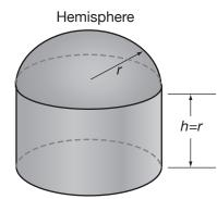
A sketch of a blind riser that is easy to cast is shown above, consisting of a cylindrical and a hemispherical portion. Note that the height of the cylindrical portion is equal to its radius (so that the total height of the riser is equal to its diameter). The volume, V, of this riser is
