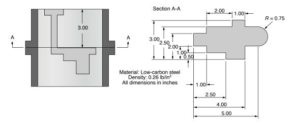
The cope mold half must be heavy enough or be weighted sufficiently to keep it from floating when the molten metal is poured into the mold. The buoyancy force, F, on the cope is exerted by the metallostatic pressure (caused by the metal in the cope above the parting line) and can be calculated using the formula
