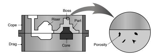
Note in the figure below that the boss is at some distance from the blind riser; consequently, the boss can develop porosity as shown because of a lack of supply of molten metal from the riser. The sketch below shows a repositioned parting line that would eliminate porosity in the boss. Note that the boss can now be supplied with molten metal as it begins to solidify and shrink.
