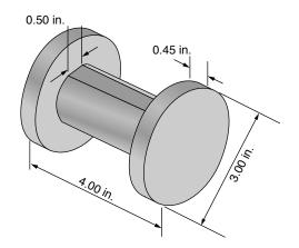
The sketch for a typical green-sand casting pattern for the spool is shown below. A crosssectional view is also provided to clearly indicate shrinkage and machining allowances, as well as the draft angles (see p. 326 for the required information). The important elements of this pattern are as follows (dimensions in inches):
