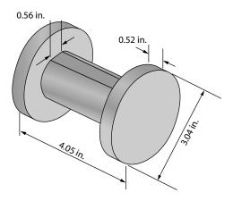
11.40 In sand casting, it is important that the cope mold half be weighted down with sufficient force to keep it from floating when the molten metal is poured in. For the casting shown in the figure below, calculate the minimum amount of weight necessary to keep the cope from floating up as the molten metal is poured in. (Hint: The buoyancy force exerted by the molten metal on the cope is dependent on the effective height of the metal head above the cope.)
