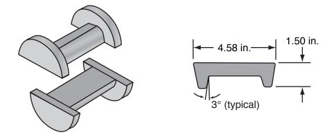
11.39 Repeat Problem 11.38 but assume that the aluminum spool is to be cast using expendable-pattern casting. Explain the important differences between the two patterns.
