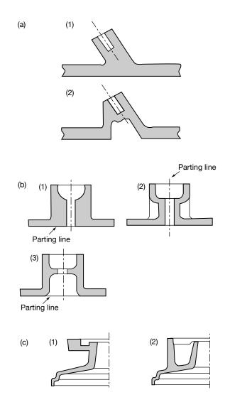
By the student. There are many observations, usually with the intent of minimizing changes in section thickness, eliminating inclined surfaces to simplify mold construction, and to orient flanges so that they can be easily cast.
