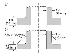
By the student. There are a number of advantages, including the fact that the part thickness is more uniform, so that large shrinkage porosity is less likely, and the ribs will control warpage due to thermal stresses as well as increase joint stiffness. This redesign illustrates the recommendations given in Figs. 12.1 and 12.2 on pp. 325-326.
