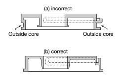
By the student. The main advantage of the new part is that it can be easily cast without using an external core. The original part requires two such cores because the shape is such that it cannot be obtained in a sand mold without using cores.
