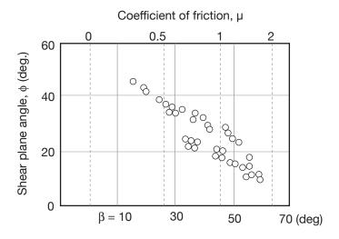
From this chart, we can estimate that for  $\beta=30^\circ$ ,  $\phi$  is approximately 25° and if  $\beta=50^circ$ ,  $\phi=15^\circ$ . We now follow the same approach as in Problem 20.41. We begin with Eq. (21.1) on p. 600 which shows the relationship between the chip thickness and depth of cut. Assume that the depth of cut and the rake angle are constant, we can rewrite this equation as
