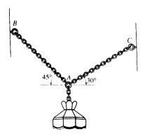
Free Body Diagram: The tension in cable AC can be determined by releasing cable AC. The system has only one degree of freedom defined by the independent coordinate  $\theta$ . When  $\theta$  undergoes a positive displacement  $\delta\theta$ , only  $\mathbf{F}_{AC}$  and the weight of lamp (10 lb force) do work.
