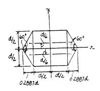
10-114. Determine the moment of inertia of the beam's cross-sectional area about the y axis which passes through the centroid C.
