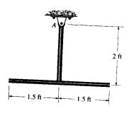
\*10-108. The pendulum consists of a plate having a weight of 12 lb and a slender rod having a weight of 4 lb. Determine the radius of gyration of the pendulum about an axis perpendicular to the page and passing through point O
