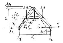
11-47. The spring attached to the mechanism has an unstretched length when  $\theta = 90^{\circ}$ . Determine the position  $\theta$  for equilibrium and investigate the stability of the mechanism at this position. Disk A is pin-connected to the frame at B and has a weight of 20 lb. Neglect the weight of the bars.
