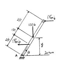
11-50. The uniform bar AB weighs 10 lb. If the attached spring is unstretched when  $\theta=90^\circ$ , use the method of virtual work and determine the angle  $\theta$  for equilibrium. Note that the spring always remains in the vertical position due to the roller guide.
