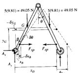
\*11-16. Determine the force F needed to lift the block having a weight of 100 lb. *Hint*: Note that the coordinates  $s_A$  and  $s_B$  can be related to the *constant* vertical length l of the cord.
