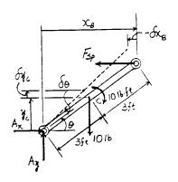
11-9. Determine the angles  $\theta$  for equilibrium of the 4-lb disk using using the principle of the virtual work. Neglect the weight of the rod. The spring is unstretched when  $\theta =$ 0° and always remains in the vertical position due to the roller guide.
