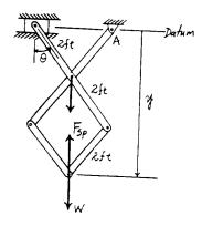
11-25. Rods AB and BC have A center of mass located at their midpoints. If all contacting surfaces are smooth and BC has a mass of 100 kg, determine the appropriate mass of AB required for equilibrium.
