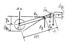
11-10. If each of the three links of the mechanism has a weight of 20 lb, determine the angle  $\theta$  for equilibrium of the spring, which due to the roller guide, always remains horizontal and is unstretched when  $\theta = 0^{\circ}$ .
