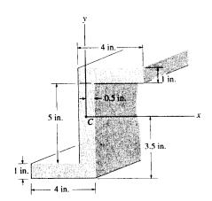
**Product of Inertia:** The area for each segment, its centroid and product of inertia with respect to x and y axes are tabulated below.
