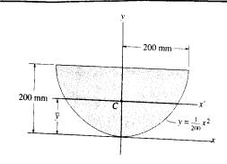
Differential Element: Here,  $x = \sqrt{200}y^{\frac{1}{4}}$ . The area of the differential element parallel to the x axis is  $dA = 2xdy = 2\sqrt{200}y^{\frac{1}{4}}dy$ .
