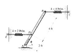
**Potential Function**: The damm is established at point A. Since the center of gravity of the beam is above the damm, its potential energy is positive. Here,  $y = (3\sin\theta)$  ft, the spring at D stretches  $x_D = (2\cos\theta)$  ft and the spring at B compresses  $x = (6\cos\theta)$  ft.
