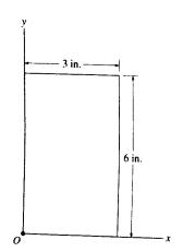
10-79. Determine the moments of inertia  $I_u$ ,  $I_v$  and the product of inertia  $I_{uv}$  of the beam's cross-sectional area. Take  $\theta = 45^{\circ}$ .
