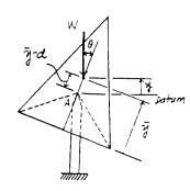
\*11-44. The triangular block of weight W rests on the smooth corners which are a distance a apart. If the block has three equal sides of length d, determine the angle  $\theta$ for equilibrium.
