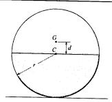
**Potential Function:** The datum is established at point A. Since the center of gravity of the cylinder is above the datum, its potential energy is positive. Here,  $y = r + d\cos\theta$ .
