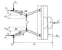
11-18. The vent plate is supported at B by a pin. If it weighs 15 lb and has a center of gravity at G, determine the stiffness k of the spring so that the plate remains in equilibrium at  $\theta = 30^{\circ}$ . The spring is unstretched when
