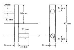
From 10-109, m = 0.1233 kg, M = 0.8478 kg, and  $\bar{I}_x = 3.25 \times 10^{-3}$ kg·m<sup>-2</sup>.
