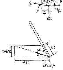
Spring Formula: From the geometry, the spring stretches  $x = \sqrt{4^2 + 1^2 - 2(4)(1)\cos 120^\circ} - \sqrt{4^2 + 1^2} = 0.4595 \text{ ft.}$
