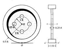
Mass Moment of Inertia About an Axis Through Point G: The mass moment of inertia of each disk about an axis passing through the center of mass can be determine using  $(I_G)_i = \frac{1}{2}mr^2$ . Applying Eq. 10-16, we have
