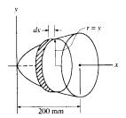
**10-95.** Determine the moment of inertia of the semiellipsoid with respect to the x axis and express the result in terms of the mass m of the semiellipsoid. The material has a constant density  $\rho$ .
