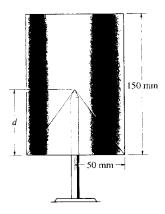
$$\bar{y} = \frac{\Sigma \bar{y} V}{\Sigma V} = \frac{75\pi (50)^2 (150) - \frac{d}{4} (\frac{1}{3}\pi) (50)^2 d}{\pi (50)^2 (150) - \frac{1}{3}\pi (50)^2 d}$$
