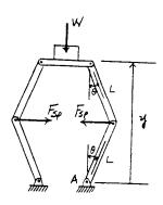
**11-31.** The two bars each have a weight of 8 lb. Determine the required stiffness k of the spring so that the two bars are in equilibrium when  $\theta = 30^{\circ}$ . The spring has an unstretched length of 1 ft.
