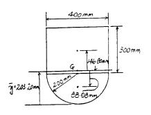
\*10-112. The pendulum consists of two slender rods AB and OC which have a mass of 3 kg/m. The thin plate has a mass of  $12 \text{ kg/m}^2$ . Determine the location  $\bar{y}$  of the center of mass G of the pendulum, then calculate the moment of inertia of the pendulum about an axis perpendicular to the page and passing through G.
