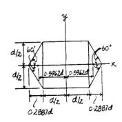
**10-115.** Determine the moment of inertia  $I_x$  of the body and express the result in terms of the total mass m of the body. The density is constant.
