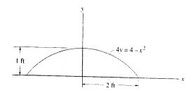
Differential Element: Here,  $y = \frac{1}{4}(4-x^2)$ . The area of the differential element parallel to the y axis is  $dA = ydx = \frac{1}{4}(4-x^2)dx$ .
