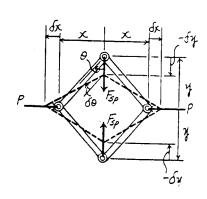
\*11-24. Determine the weight W of the crate if the angle  $\theta = 45^{\circ}$ . The springs are unstretched when  $\theta = 60^{\circ}$ . Neglect the weights of the members.
