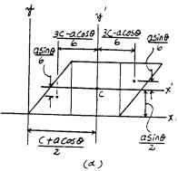
10-71. Determine the product of inertia of the cross sectional area with respect to the x and y axes.
