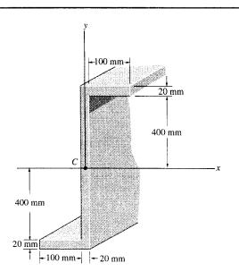
\*10-72. Determine the product of inertia of the beam's cross-sectional area with respect to the x and y axes that have their origin located at the centroid C.
