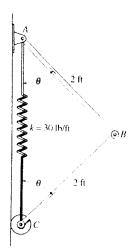
**Potential Function:** The datum is established at point A. Since the center of gravity of the bars are below the datum, their potential energy is negative. Here,  $y_1 = 1\cos\theta$  ft,  $y_2 = 2\cos\theta + 1\cos\theta = 3\cos\theta$  ft and the spring stretches  $x = 2(2\cos\theta) - 1 = (4\cos\theta - 1)$  ft.
