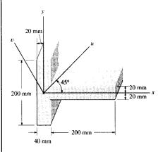
Moment and Product of Inertia about x and y Axes: Since the shaded area is symmetrical about the x axis,  $I_{\rm xy}=0$ .
