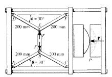
**Free Body Diagram:** The system has only one degree of freedom defined by the independent coordinate  $\theta$ . When  $\theta$  undergoes a positive displacement  $\delta\theta$ , only the forces  ${\bf F}$  and  ${\bf P}$  do work.
