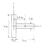
10-78. Determine the directions of the principal axes with origin located at point O, and the principal moments of inertia for the rectangular area about these axes.
