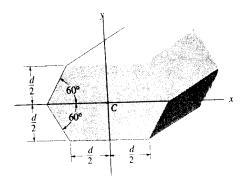
Moment of Inertia: The moment of inertia about the x axis for the composite beam's cross section can be determined using the parallel – axis theorem  $I_x = \Sigma \left(\bar{I}_x + A d_y^2\right)_i$ .
