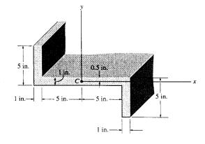
10-73. Determine the product of inertia for the angle with respect to the x and y axes passing through the centroid C. Assume all corners to be square.
