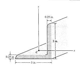
10-74. Determine the product of inertia for the beam's cross-sectional area with respect to the u and v axes.
