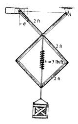
**Potential Function**: The damm is established at point A. Since the center of gravity of the crate is below the damm, its potential energy is negative. Here,  $y = (4\sin\theta + 2\sin\theta) = 6\sin\theta$  ft and the spring stretches  $x = 2(2\sin\theta - 2\sin 30^\circ) = (4\sin\theta - 2)$  ft.
