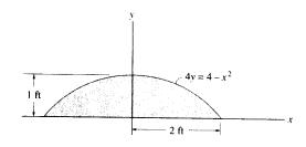
**Differential Element:** Here,  $y = \frac{1}{4}(4-x^2)$ . The area of the differential element parallel to the y axis is dA = ydx. The moment of inertia of this differential element about the x axis is
