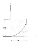
**Differential Element:** Here,  $x = y^{\frac{1}{3}}$ . The area of the differential element parallel to the x axis is  $dA = xdy = y^{\frac{1}{3}}dy$ . The coordinates of the centroid for this element are  $\tilde{x} = \frac{x}{2} = \frac{1}{2}y^{\frac{1}{3}}$ ,  $\tilde{y} = y$ . Then the product of inertia for this element i.
