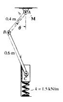
Free Body Diagram: The system has only one degree of freedom defined by the independent coordinate  $\theta$ . When  $\theta$  undergoes a positive displacement  $\delta\theta$ , only the spring force  $F_{sp}$  and couple moment M do work.
