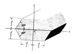
Moment of Inertia: The moment of inertia about yaxis for the composite beam's cross section can be determined using the parallel – axis theorem  $I_y = \Sigma \left( \bar{I}_y + A d_x^2 \right)_i$ .
