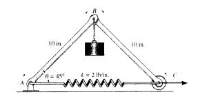
**Free Body Diagram**: The system has only one degree of freedom defined by the independent coordinate  $\theta$ . When  $\theta$  undergoes a positive displacement  $\delta\theta$ , only the spring force  $F_{ip}$ , the weight of links (2 lb), 20 lb force and force **P** do work.
