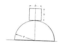
Potential Function: The damm is established at point O. Since the center of gravity for the block is above the datum, its potential energy is positive. Here,  $y = \left(r + \frac{b}{2}\right)\cos\theta + r\theta\sin\theta$
