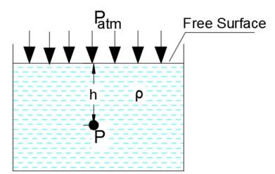
As shown in figure above, distance z is measured from the free surface  $\rightarrow z = -h \rightarrow P = \rho gh + constant.$
