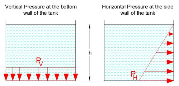
As shown in figure above, a tank contains water and the vertical pressure at depth (h) is  $P_V$  and it's applied on the bottom wall of the tank.
