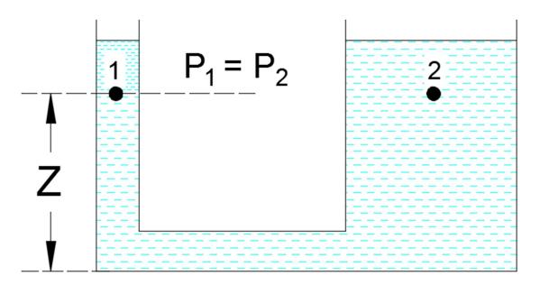
Note that the conditions are satisfied (continuous fluid and same fluid), so the pressure at points 1 and 2 is equal. But the **forces** at points 1 and 2 are not equal because the area at point 1 doesn't equal the area at point 2.
